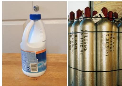
*1/3 gallon of 7.5% strength chlorine bleach (left) and 150 lb. cylinders of liquefied chlorine (right). Chlorine cylinder photo courtesy of [The Chlorine Institute](#).*
