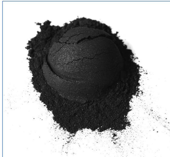
*Activated carbon is used by water treatment facilities to help improve water quality. Many home water treatment devices also employ activated carbon, especially to help reduce water odor and taste.*
